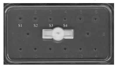
**Figure 2.** Determining the concentration of colostral IgG with radial immunodiffusion (RID) assay. Wells 1-4, S1-S4: Standard IgG samples containing 2.5, 1.25, 0.62, and 0.31 g/L IgG respectively. Wells 5-14: Diluted colostrum samples.
